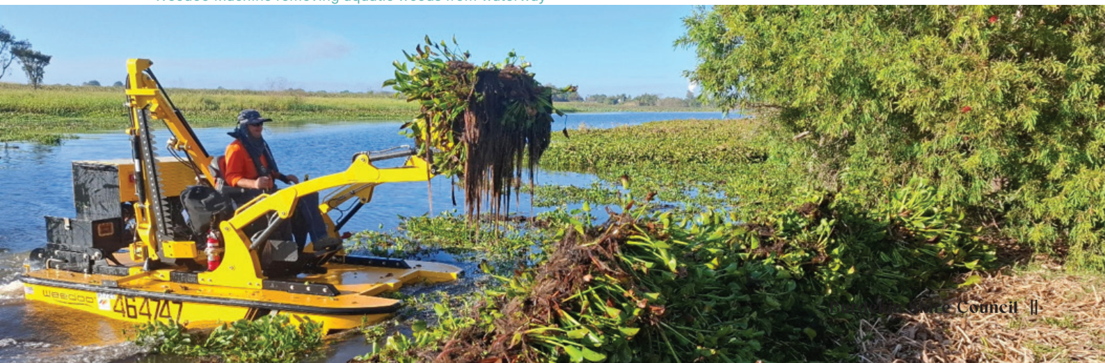
📍 Weedoo Machine removing aquatic weeds from waterway
