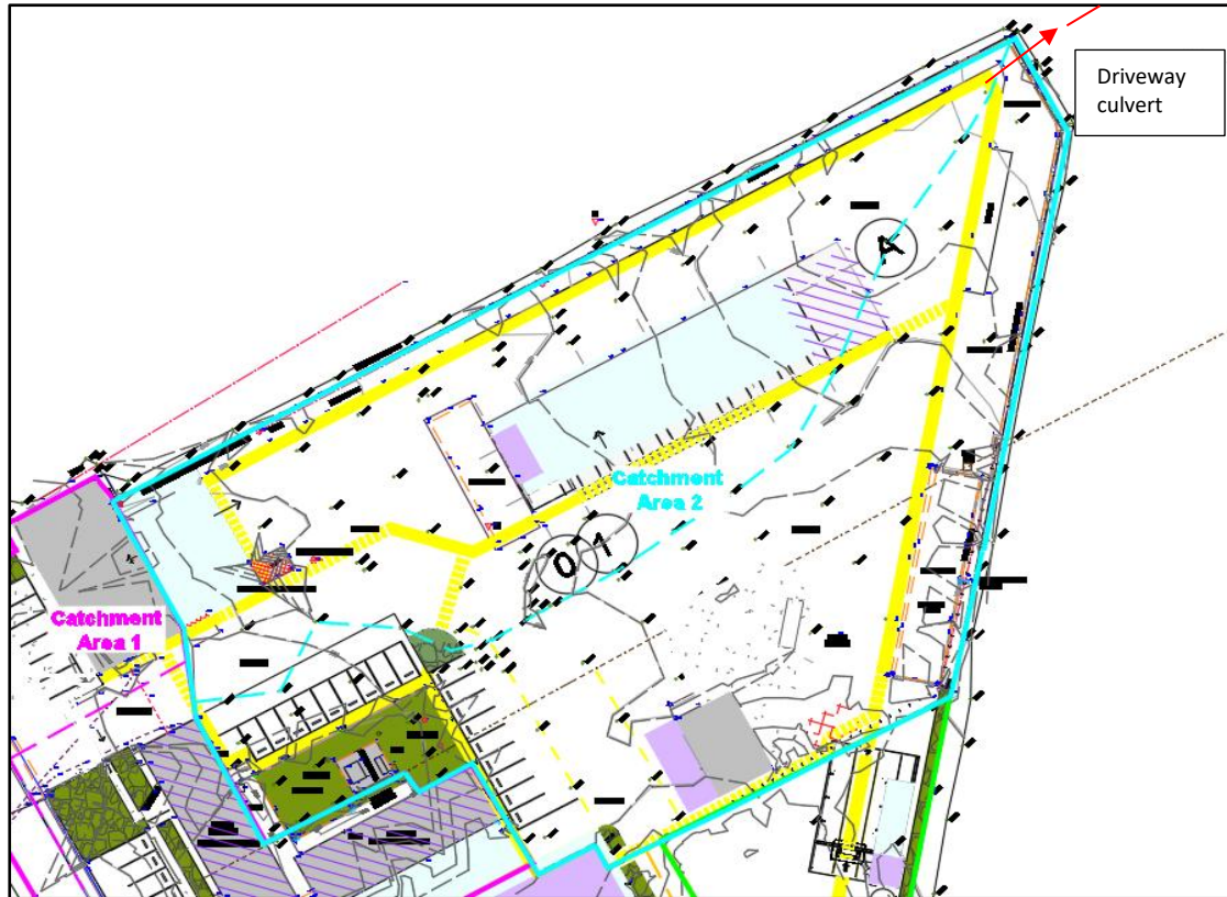
Figure 15 : Proposed culvert catchment area
