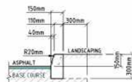
BARRIER KERB (BK) TYPICAL DETAIL - SCALE 1:20 @ A1
