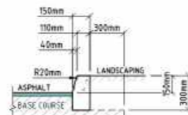
BARRIER KERB (BK) TYPICAL DETAIL - SCALE 1:20 @ A1
