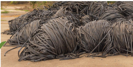
CORRECT: Neatly bound, contaminant free rolls
